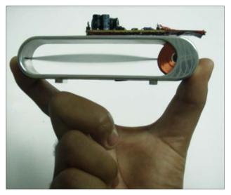
The µicroWindbelt™ uses aeroelastic flutter & vibration rather than a spinning turbine to make micro-wind harvesting possible at 10x the efficiency of turbine-based approaches (Nature. Priya Nov. 8, 2005)
